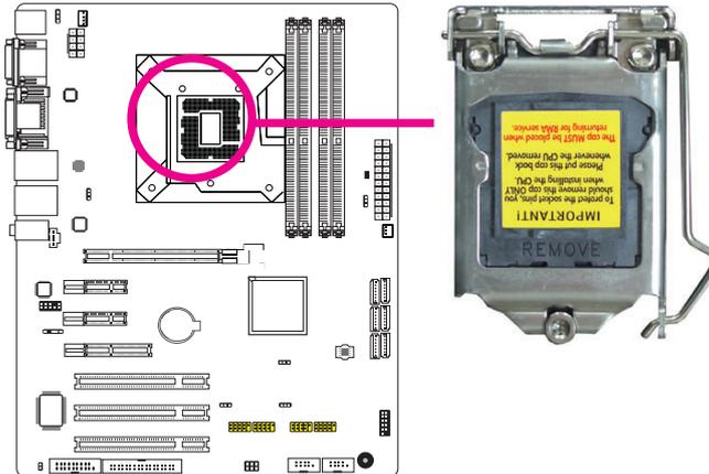
4. Unlock the socket by pushing the load lever down, moving it sideways until it is released from the retention tab; then lift the load lever up.
