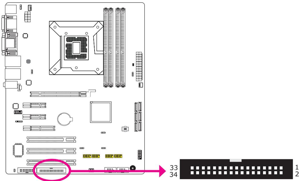
The FDD connector supports a standard floppy disk drive. The floppy cable can be inserted into this connector only if pin 1 of the cable is aligned with pin 1 of this connector.
