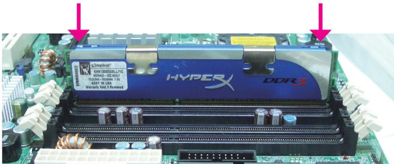
8. The ejector tabs at the ends of the socket will automatically snap into the locked position to hold the module in place.
