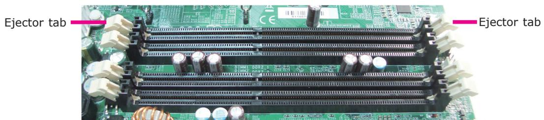
5. Note how the module is keyed to the socket.
