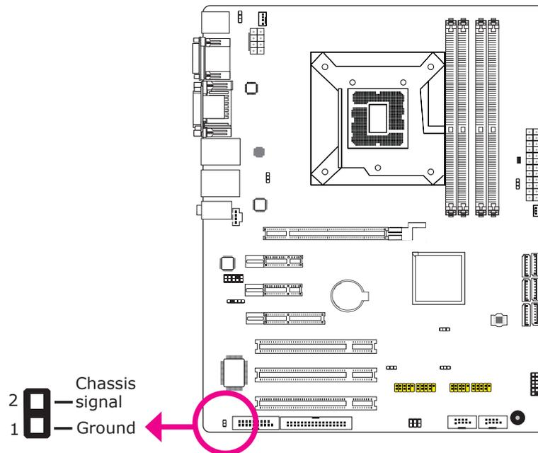
The board supports the chassis intrusion detection function. Connect the chassis intrusion sensor cable from the chassis to this connector. When the system's power is on and a chassis intrusion occurred, an alarm will sound. When the system's power is off and a chassis intrusion occurred, the alarm will sound only when the system restarts.
