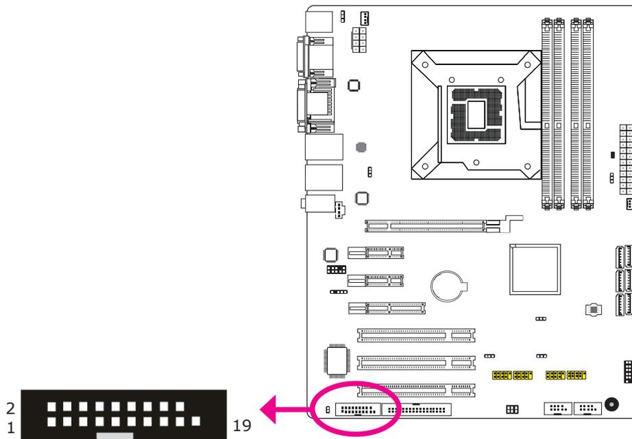
The Digital I/O connector provides powering-on function to an external device that is connected to this connector.
