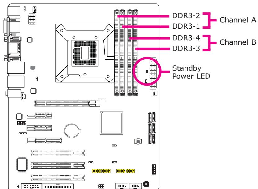
The four DIMM sockets are divided into 2 channels:
