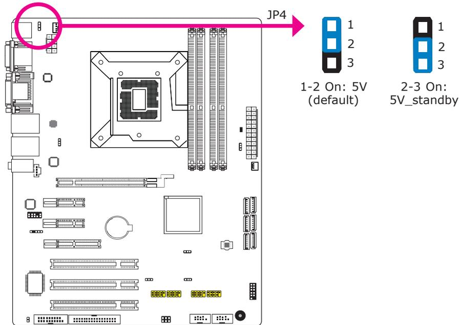
JP4 is used to select the power of the PS/2 keyboard/mouse port. Selecting 5V\_standby will allow you to use the PS/2 keyboard or PS/2 mouse to wake up the system.
