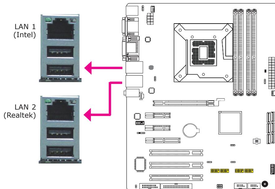
The LAN ports allow the system board to connect to a local area network by means of a network hub.
