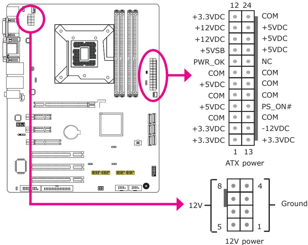
Use a power supply that complies with the ATX12V Power Supply Design Guide Version 1.1. An ATX12V power supply unit has a standard 24-pin ATX main power connector that must be inserted into the 24-pin connector. The 8-pin +12V power connector enables the delivery of more +12VDC current to the processor's Voltage Regulator Module (VRM).
