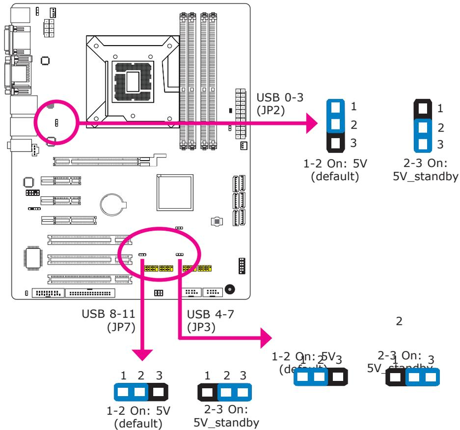
These jumpers are used to select the power of the USB ports. Selecting 5V\_standby will allow you to use a USB device to wake up the system.
