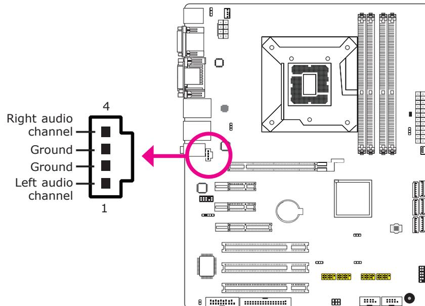
The CD-in connector is used to receive audio from a CD-ROM drive, TV tuner or MPEG card.
