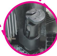
"Unlocked" position of push-pin
